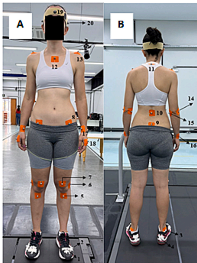
Fig. 1. Marker model used for collecting running biomechanics data: 1 – head of the second metatarsal; 2 – head of the fifth metatarsal; 3 – lateral malleolus; 4 – calcaneus; 5 – tibial tuberosity; 6 – lateral epicondyle of the femur; 7 – patella (1 cm above the superior border of the patella); 8 – anterior superior iliac spine; 9 – sacrum (midpoint between the left and right posterior superior iliac spines); 10 – spinous process of the twelfth thoracic vertebra (T12); 11 – spinous process of the second thoracic vertebra (T2); 12 – jugular notch; 13 – acromion; 14 – lateral epicondyle of the humerus; 15 – medial epicondyle of the humerus; 16 – styloid process of the ulna; 17 – styloid process of the radius; 18 – base of the index finger; 19 – glabella; 20 – tragus of the ear. A – anterior view; B – posterior view.
